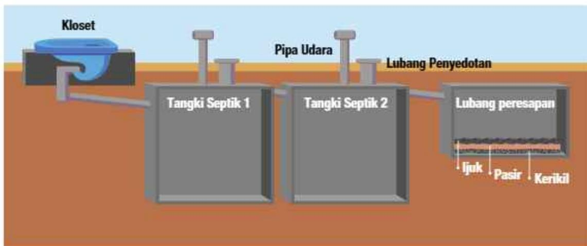
Gambar 2. *Septic Tank* 2 Chamber
