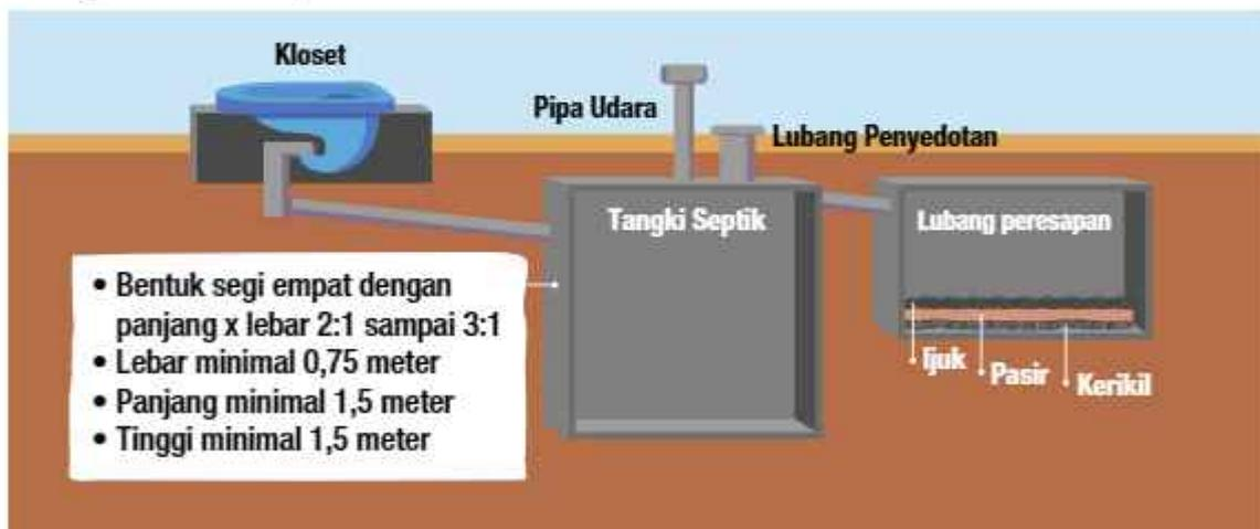
Gambar 1. *Septic Tank* 1 Chamber
